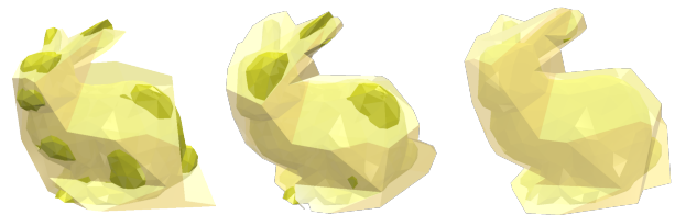
Figure 11: Examples of over-cuts as captured by the 3D scanner (left and middle). Offsetting the instructions helped in reducing them (right model).
