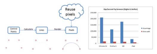
Using pixel cashing is more than ten-times faster than normally drawing the path [15]
