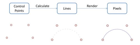
Figure 3 Flattening and rendering Bézier curve
